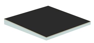
The tapered rigid insulation panels are tailor-made by Millenium according to dimensions and slope specifications. They are composed of type 1 or 2 expanded polystyrene [EPS] rigid insulation, laminated in the factory to a 13 mm wood fiber board to meet the various requirements of projects.
