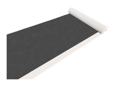
The Millenium Vapour Protector Membrane is made of SBS modified bitumen with a non-woven glass fiber mat. It is specially designed to be installed before the installation of thermal insulation and the roofing membrane.
